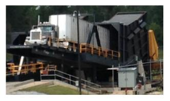
Delivery of the wood: The specialized woodchip trucks are weighed then backed onto one of the two truck tippers. A sample of the woodchips is taken to ensure quality. Then the whole truck is tipped so that the chips fall out of the back of the truck. Very interesting! If the wood is wet, the chips will be spread out on the back part of the lot for drying by the sun.
